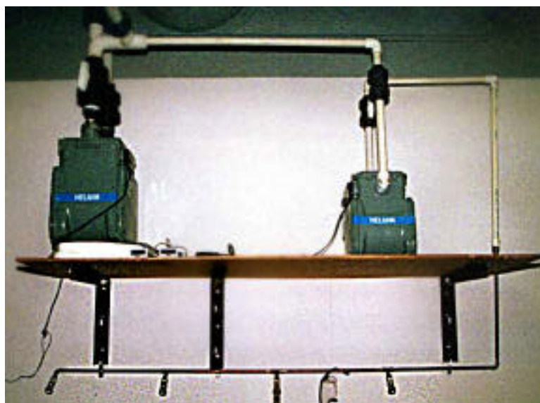
Ballast tank with compressors. Gas bag to right. Cost of equipment in room - approximately $5000.
