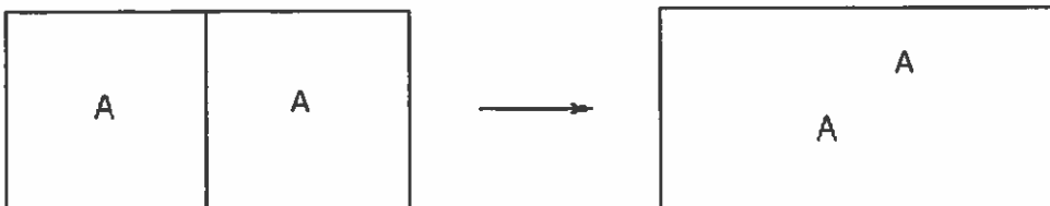
Figure 2. Shows the result of combining two identical gases after the partition is removed. The total entropy change is equal to zero.
