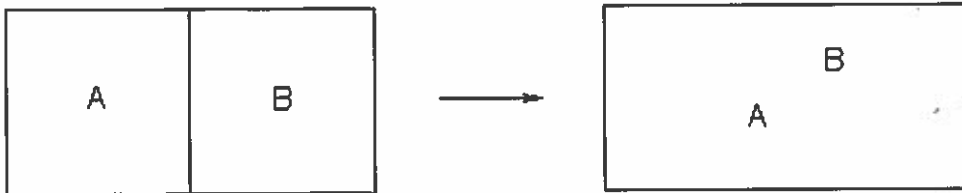
Figure 1. Shows two different gasses initially separated by a partition then combined after the removal of the partition.
